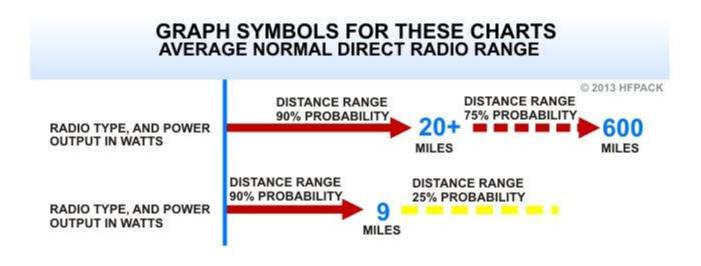
The above graph shows the distance range between two base stations using a basic antenna mounted on the roof of a suburban house with a height of about 20ft above ground level. Communication distance can be greatly improved over this by advanced gain antenna systems or a high pole or a tower. This estimate is based upon radio-to-radio direct communications without the use of a repeater.
